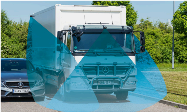
The modular SurroundView system merges recordings of the surroundings together onto one monitor, allowing blind spots to be viewed.
