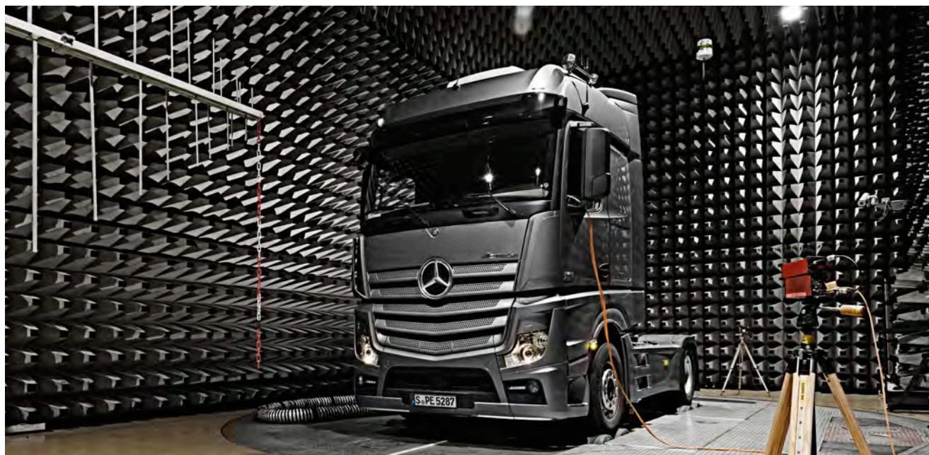
EMC test in a laboratory that is especially shielded against external electromagnetic interferences.
